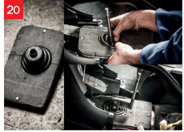
To keep noise and harshness out of the cabin, the boys made up a custom gear surround. Made from a fibreglass plate covered in Dynamat, it includes a generic rubber boot to grip the gearstick, minimizing any unwanted noise that may reach the cabin from beneath the car.
