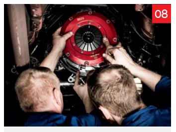
With the flywheel mounted, the clutch alignment tool comes into play to ensure that the friction disc(s) are centred. Push it through the splined centre hole in the friction disc and locate it in the spigot bush. The pressure plate can now be bolted onto the flywheel. Again, it is critical that the correct torque settings are used.
