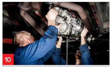
The fun part of fitting the manual gearbox can now begin. The Gearbox Factory prefers to perform manual conversions with the engine still in the car to avoid the time and hassle of first removing, then reinstalling it. Though this throws in the challenge of fastening the upper bellhousing bolts (attaching the bellhousing to the engine block), this is not normally a problem given patience and dextrous hands.
