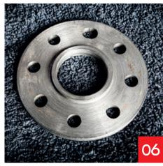
This spacer was made to fit between the crankshaft and the flywheel, ensuring that the starter motor correctly engages the ring gear on the aftermarket flywheel. In this case, the starter motor was able to be reused, although it is always advisable to check first whether a different starter motor will be required.
