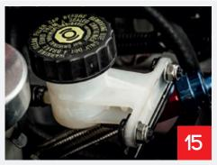
The clutch master cylinder used here is a reconditioned second-hand unit from a latemodel manual Commodore. Some cars will have master cylinders available off-theshelf; others may require one from a different application be made to fit. Most cars that came out of the factory with a manual option have a mark on the firewall (it may be on the inside of the firewall)
